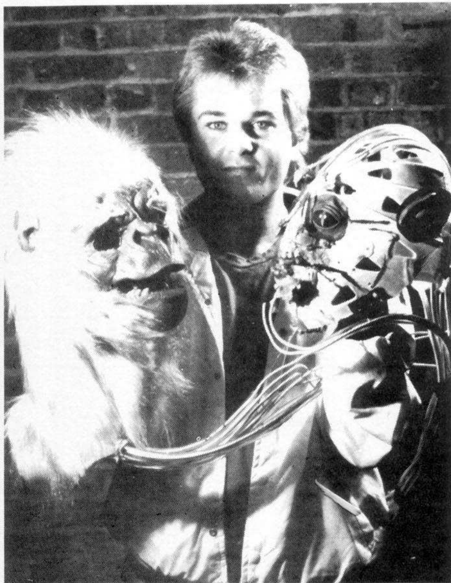
Arnold Gargiulo and his handiwork. Shown here are two wearable masks (one under construction) with faces that move. Note the control cables and the goalie mask construction of the uncompleted mask on the right.
